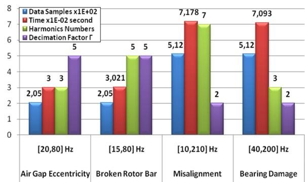
Figure 13. Computation time depending on Fault Frequency range and decimation factor
