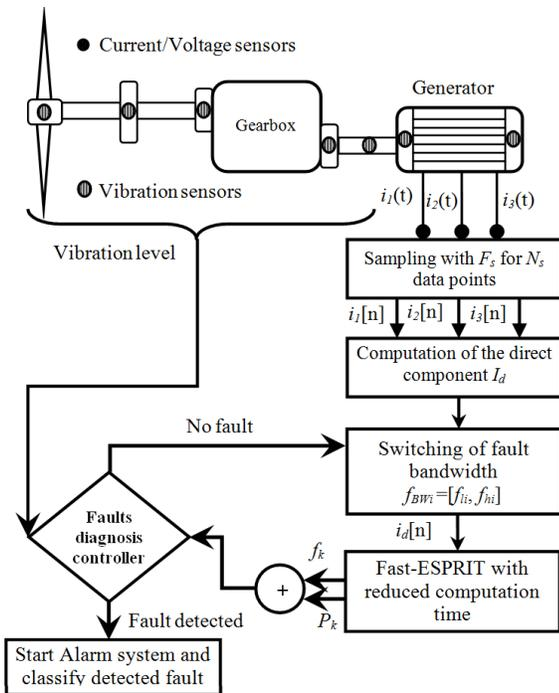
Figure 3. Intelligent wind turbine faults diagnosis by Fast-ESPRIT.
