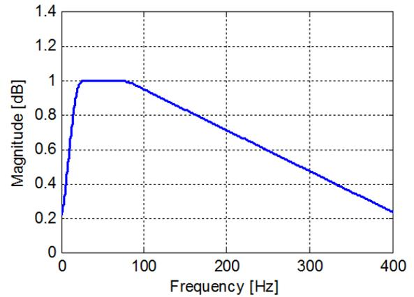
**Figure 5.** IIR filter Yule-Walk frequency response gain.
