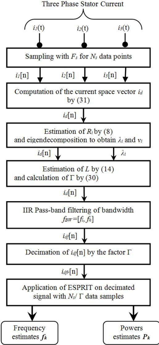
Figure 1. Block diagram scheme of the Fast-ESPRIT algorithm.
