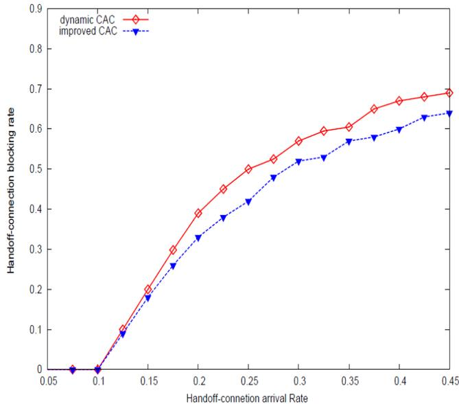
**Figure 3.** Dropping rates of handoff connections with the traffic rates of 1:1.
