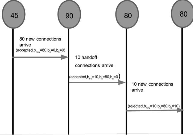
**Figure 1.** The process of connection admissions with the dynamic CAC and BR scheme
